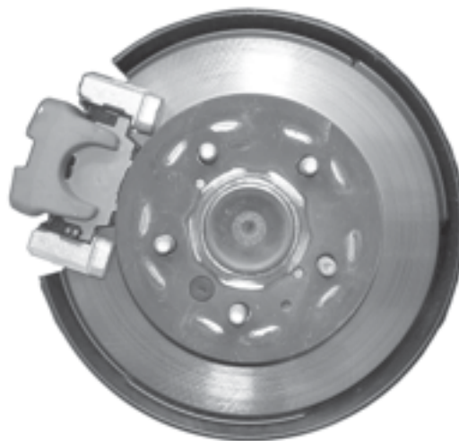
Rear Brake Caliper & Disc
